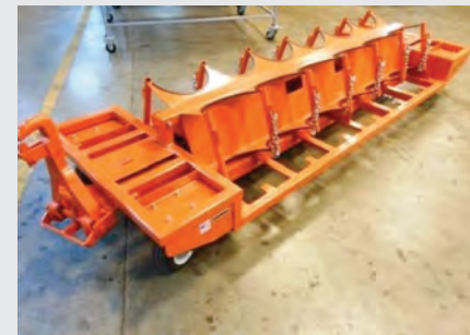
Link Caster Steer Industrial Trailer for transporting cylinders.
